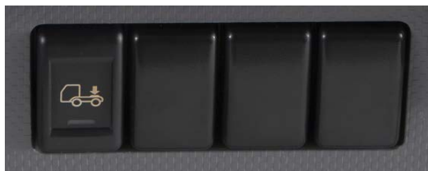
Figure 11 - Dump/Fill Toggle Switch
