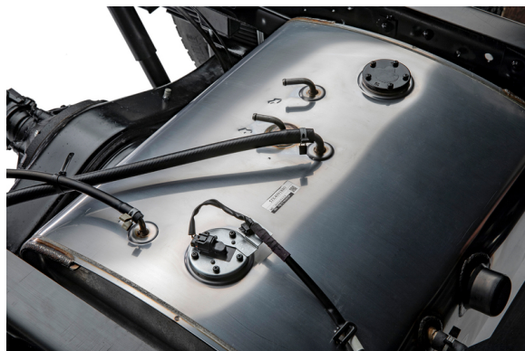
Figure 14: N-Series Standard Stainless Steel Fuel Tank
